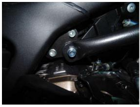
Slide the rear arm of the crashbar over the bolt and screw on the supplied nut, but do not tighten fully.
