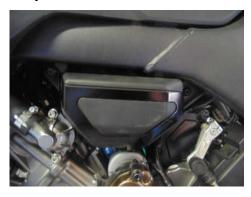
Remove the toolbox by undoing the two bolts under the frame.
