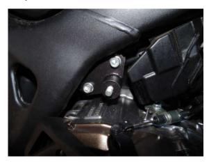
Attach the right bracket to the motorcycle, using the spacers from the previous bracket, along with the bolts.
