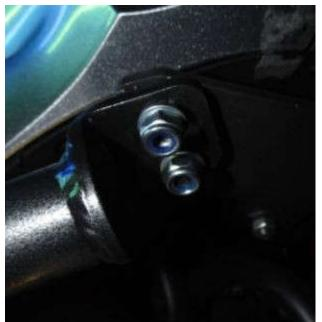
Using two bolts attach the front of the crashbar
