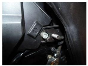
Insert the left bracket with the bolt going through the motorcycle
