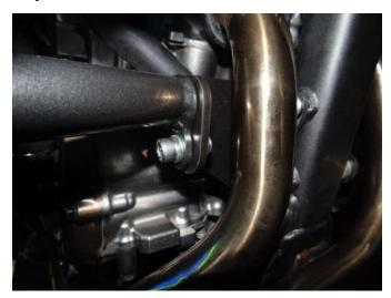
Fit the bottom of the crashbar to the engine brackets using the bolts supplied.
