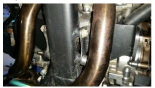
Fix the bottom brackets to the frame using the bolts supplied along with the 10mm Aluminium spacer on the left.
